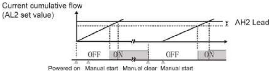
★ AH2 means control output lead value.
