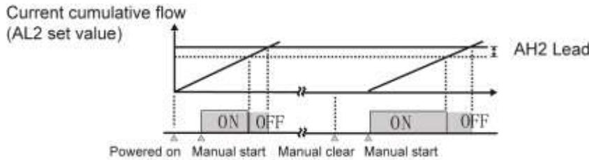
★ AL2 quantitative control output: (manually start the output of "0")
